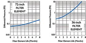
As the solid particles traveling in the gas stream accumulate on the filter elements over time, the differential pressure will increase due to the restriction of gas flow. The diagrams illustrate the comparison of 36-inch and 72-inch filter element lengths in terms of element life.
