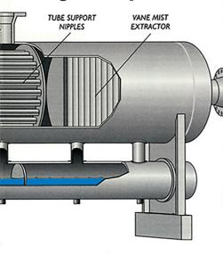
enough to drop out once the velocity is reduced inside the vessel. This liquid is conveniently drained into the first section of the sump to eliminate its passing through the filter elements. Solid particles collected by the filter elements will eventually begin to restrict the gas flow. When the resulting pressure drop reaches 10 PSI or 10% of system pressure, the filter elements should be changed.
